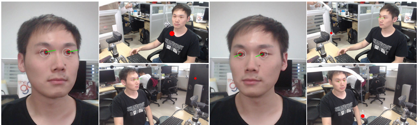
Figure 1: We present a real-time 3D gaze tracking method using a single consumer-level RGB camera, without the use of any infra-red illuminators. The estimated 3D gaze target is visualized as a red point from two additional views, which are not used for actual tracking. Our novel calibration method is “ground-truth position free”, allowing for deployment in a diverse array of application scenarios.
